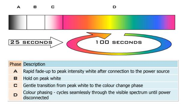
**Freezing the colour:** The stand-alone programme may be halted at any time by briefly switching the power supply *off* and then back *on* again (within less than a second). This simple action allows the light source to be frozen on any particular colour (or white) just by toggling the switch controlling power to the device.
